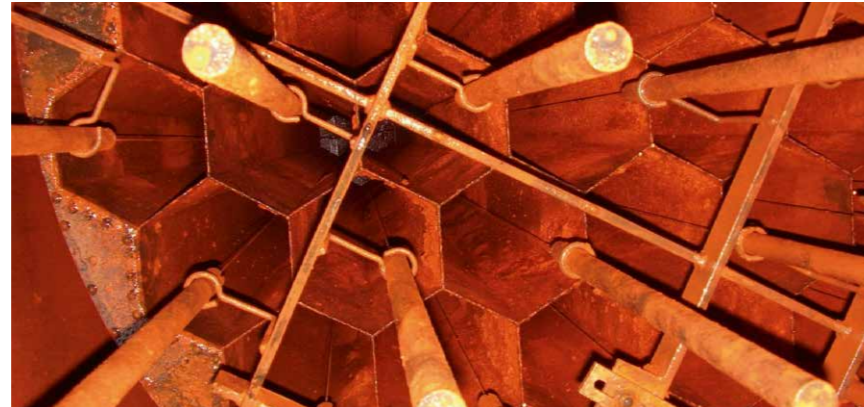
Honeycombs of a wet electrostatic filter
