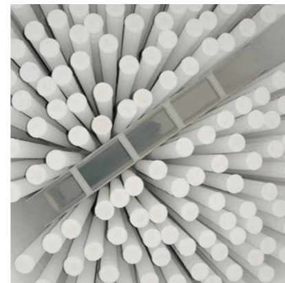
Hose filter, raw gas side
